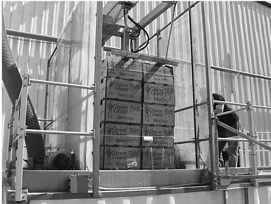
The Deepchill system lowers an entire pallet of waxed boxes into a stainless steel chamber containing a mix of ice crystals and water. After one minute, the pallet is removed. Water drains out of the boxes, leaving the ice behind.
